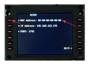
In the same way, using the FMC keyboard, change the MAC address, by adding a single number:02-00-00-00-01 should be good, because in a networked multi CDU system the mac address of every CDU must be unique, confirm with LSK-1. Please note: the first number of Mac address must remain "02".
