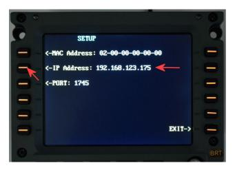
After a few seconds, the "SETUP" screen on the left will be displayed, if not, unplug the power cable an repeat.
